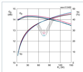
$V_{DS}$  = 28 V;  $I_{Dq}$  = 1000 mA;  $V_{GS(amp)peak}$  = 0.50 V.
