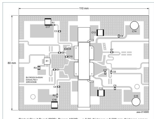
Printed-Circuit Board (PCB): Rogers 4350B:  $\epsilon_r$  = 3.66; thickness = 0.508 mm; thickness copper plating = 35  $\mu$ m. See Table 16 for a list of components.
