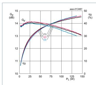
$V_{DS} = 28 \text{ V}; I_{Dq} = 1000 \text{ mA}; V_{GS(amp)peak} = 0.50 \text{ V}.$
